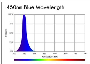
The 450nm wavelength is recommended as supplemental light for seedlings and young plants during the vegetative stage of their growth cycle, especially when "stretching" must be reduced or eliminated.
