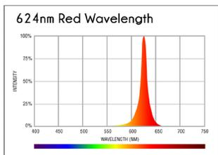
This 624nm region has the highest photosynthetic relative quantum yield for a range of plants. Its action on red-absorbing phytochrome is considerably weaker compared to that of 660nm red light.
