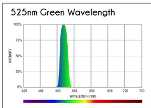
The 525nm wavelength LED can be used as a tool for eliciting specific plant responses such as stomatal control, phototropism, photomorphogenic growth and environmental signaling.
